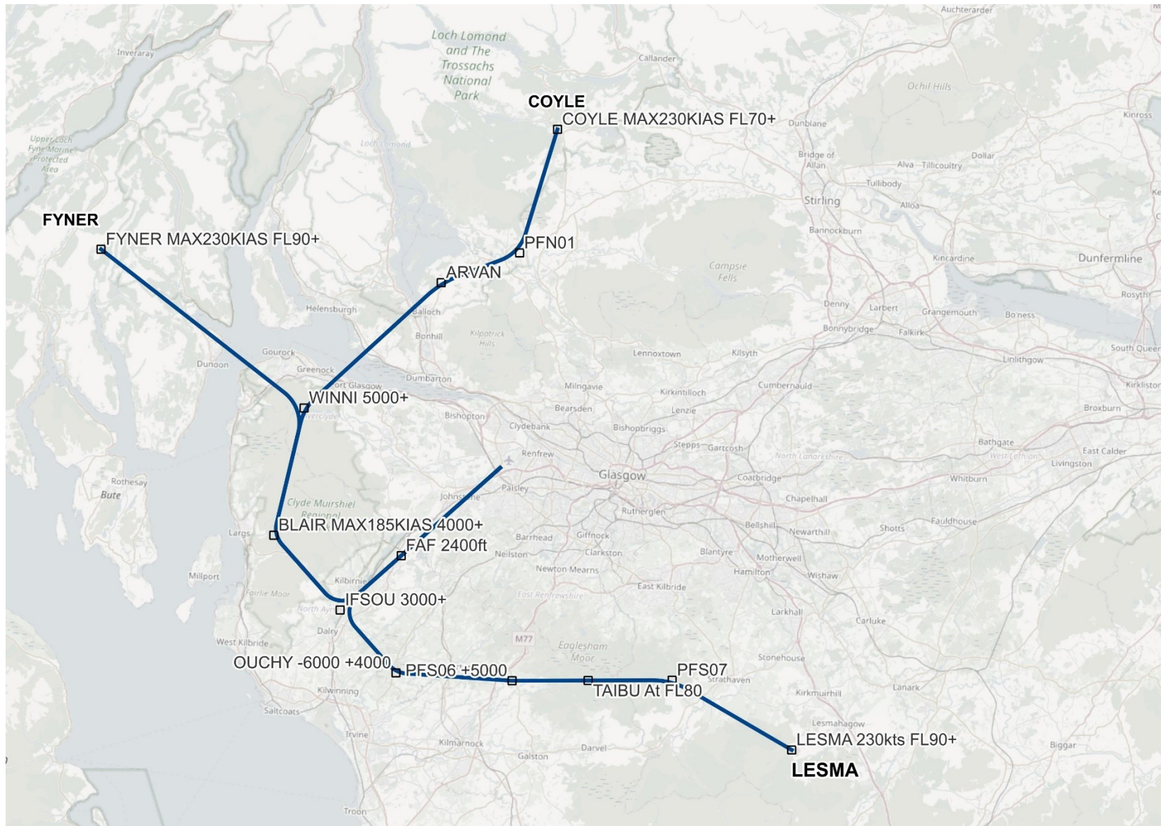
Figure 8 Runway 05 RNAV 1 (DME/DME or GNSS) arrival transitions and approach procedures (does not show missed approach procedures)
