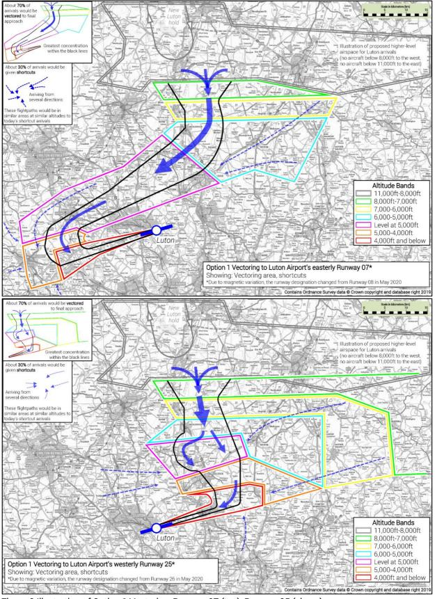
Figure 3 Illustration of Option 1 Vectoring, Runway 07 (top), Runway 25 (above)
