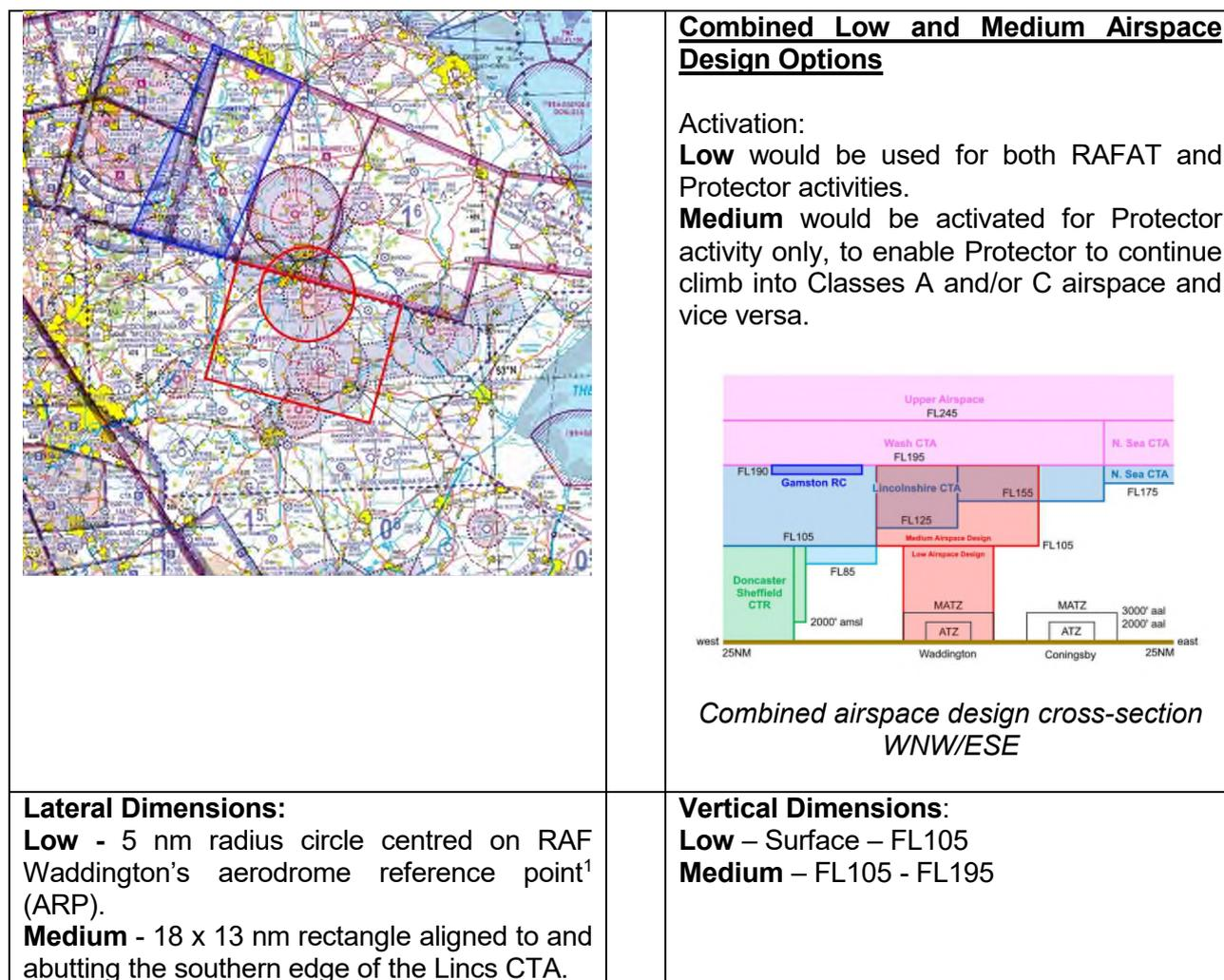
Figure 1- Combined Low and Medium airspace designs
