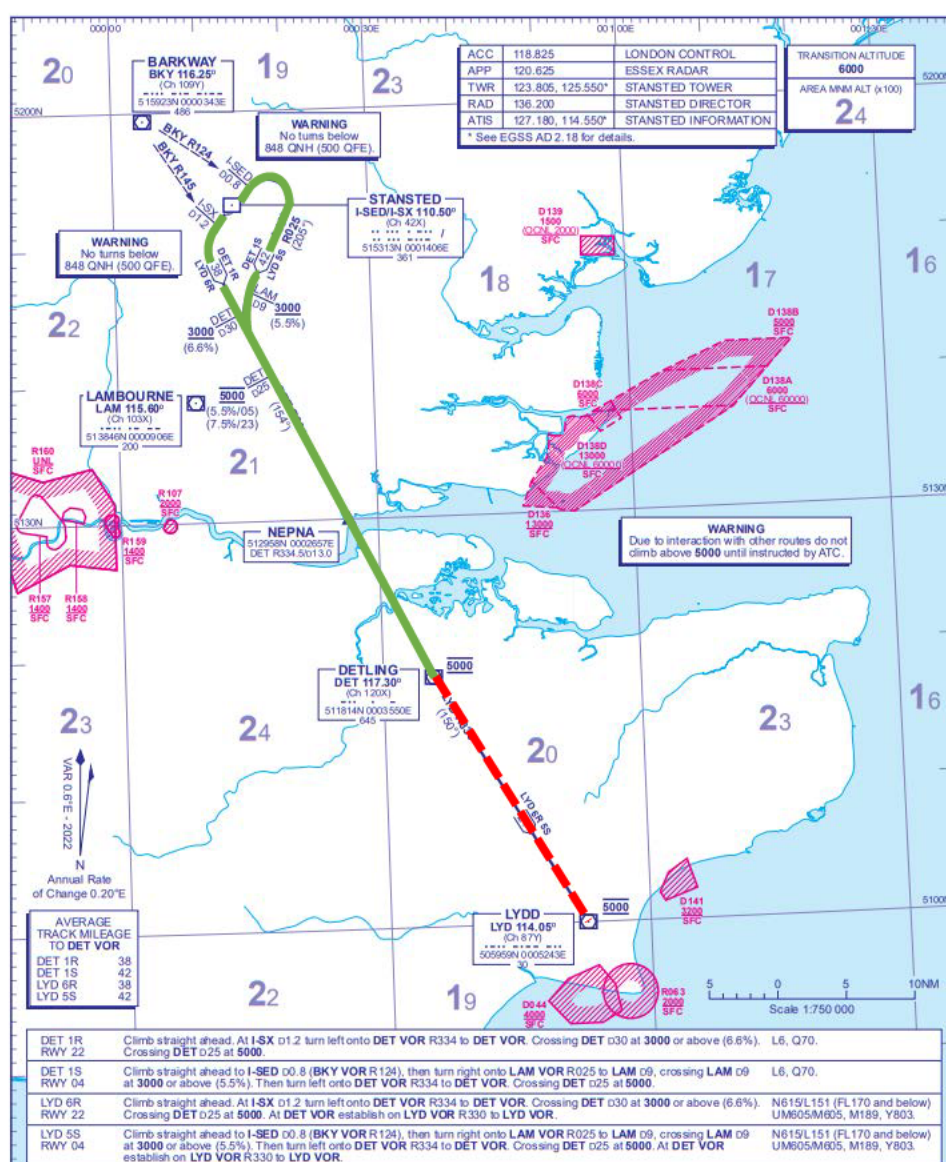
Figure 4: Proposed routing for South East Departures. Aircraft will fly the DET 1R/1S SIDs (green line) to DET before continuing onto the extended M604 (red dashed line) to join ATS route network.
