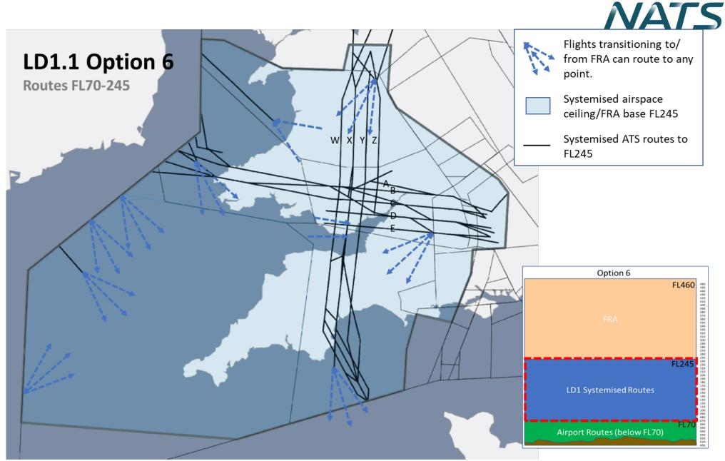
Figure 8 Option 6: Systemised routes FL70-245, with indicative FRA transitions from FL245
