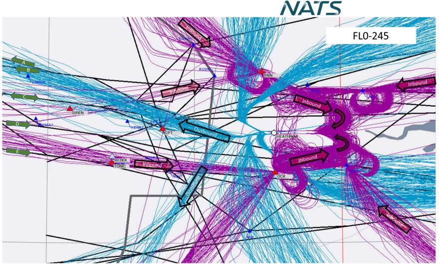
Figure 53 LTMA interface. Extant Heathrow Arrivals & Departures and proposed route structure (1 week – Aug 2019 data, below FL245, arrivals purple and departures blue) (note a separate pdf giving these trajectories layered by altitude is included in consultation materials. This allows you to assess the typical altitude of overflight in a particular location).
