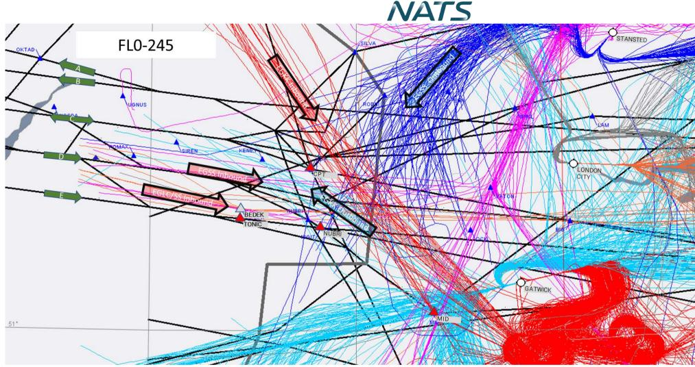
Figure 55 LTMA interface. Extant Stansted, Gatwick, London City Arrivals & Departures and proposed route structure (1 week – Aug 2019 data, below FL245, arrivals pink/red and departures blue/grey) (note a separate pdf giving these trajectories layered by altitude is included in consultation materials.)
