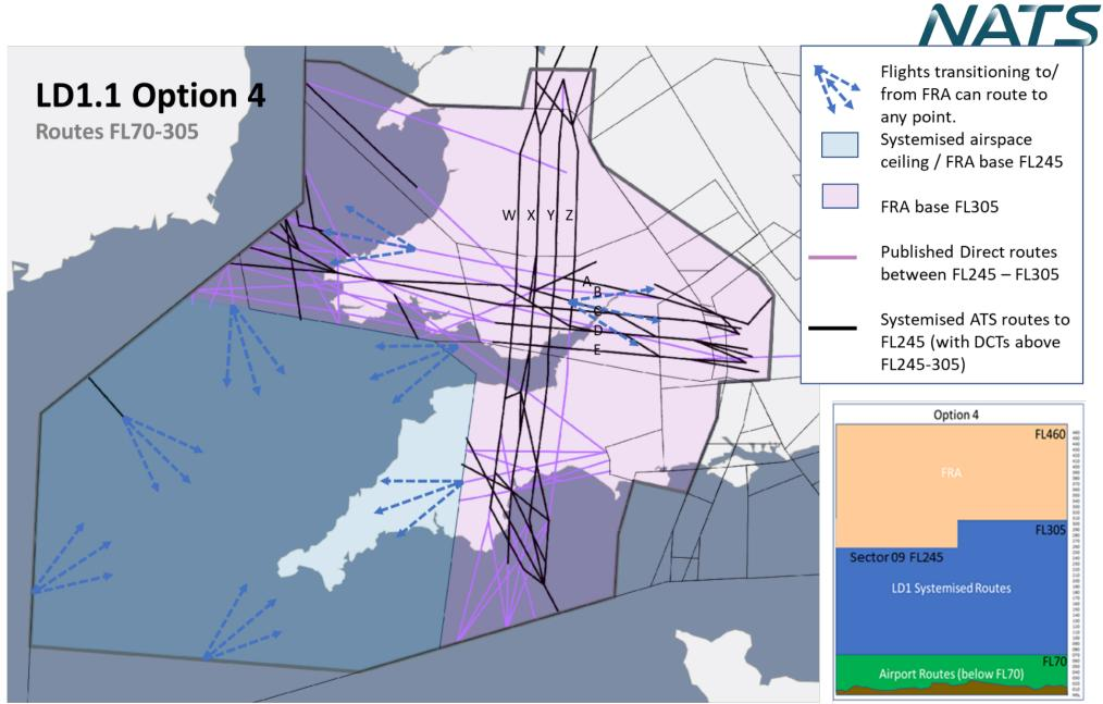
Figure 7 Option 4: Change to systemised routes FL70-305 with indicative FRA transitions
