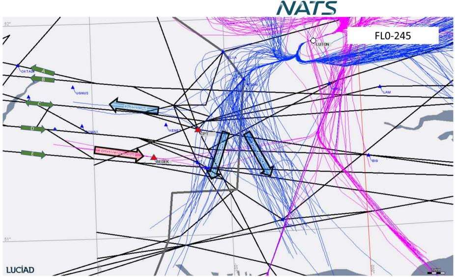
Figure 54 LTMA interface. Extant (2019) Luton Arrivals & Departures and proposed route structure (1 week – Aug 2019 data, below FL245, arrivals pink and departures blue) (note a separate pdf giving these trajectories layered by altitude is included in consultation materials. This allows you to assess the typical altitude of overflight in a particular location)
