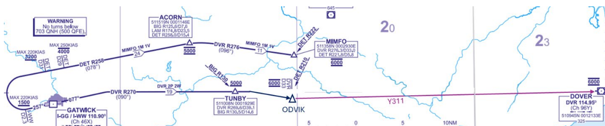
Figure 12 - Proposed DVR SID and ATS connectivity (purple arrow). Source: Adapted from UK AIP London Gatwick AD2.24 07.04.2026
