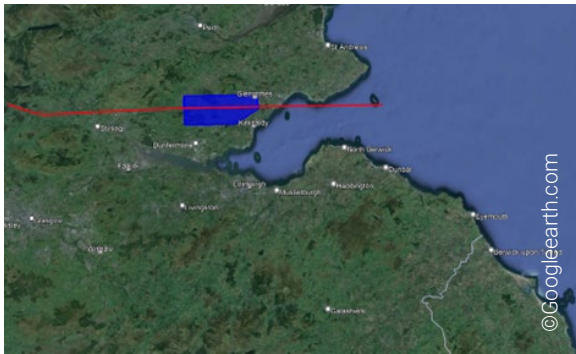
Figure 39: ScTMA 6 (blue shape) location. ATS routes are shown in yellow, STARs in red, holds in green, transitions in white and SIDs in orange.
