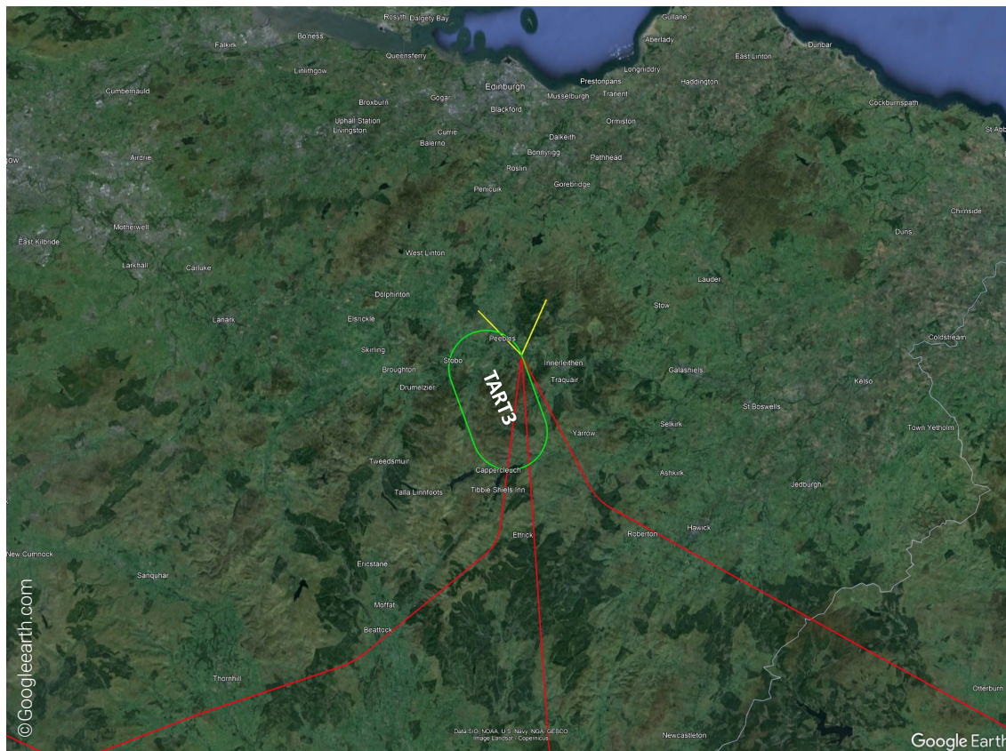
Figure 29: Location of proposed TART3 hold (green line) and associated STARs (red lines) and arrival transition above 7,000 ft (yellow lines).
