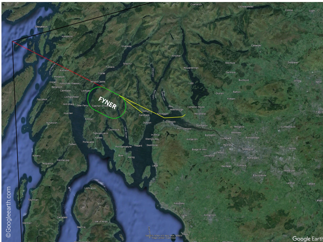
Figure 30: Location of proposed FYNER hold (green line) and associated STARs (red line) and arrival transition above 7,000 ft (yellow lines).
