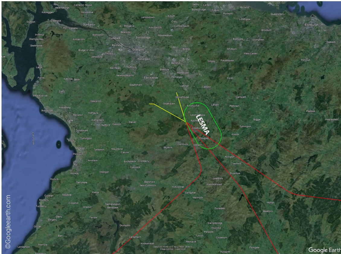
Figure 32: Location of proposed LESMA hold (green line) and associated STARs (red lines) and arrival transition above 7,000 ft (yellow lines).
