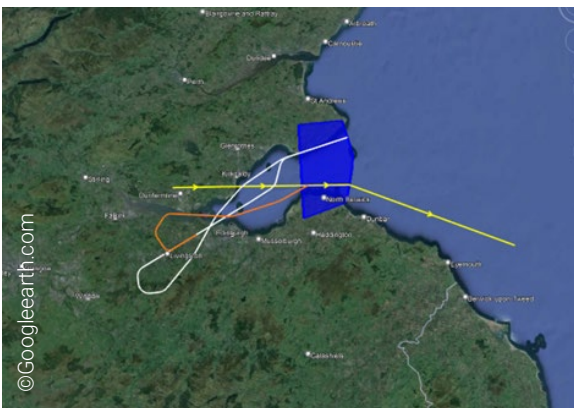
Figure 38: ScTMA 5 (blue shape) location. ATS routes are shown in yellow, STARs in red, holds in green, transitions in white and SIDs in orange.
