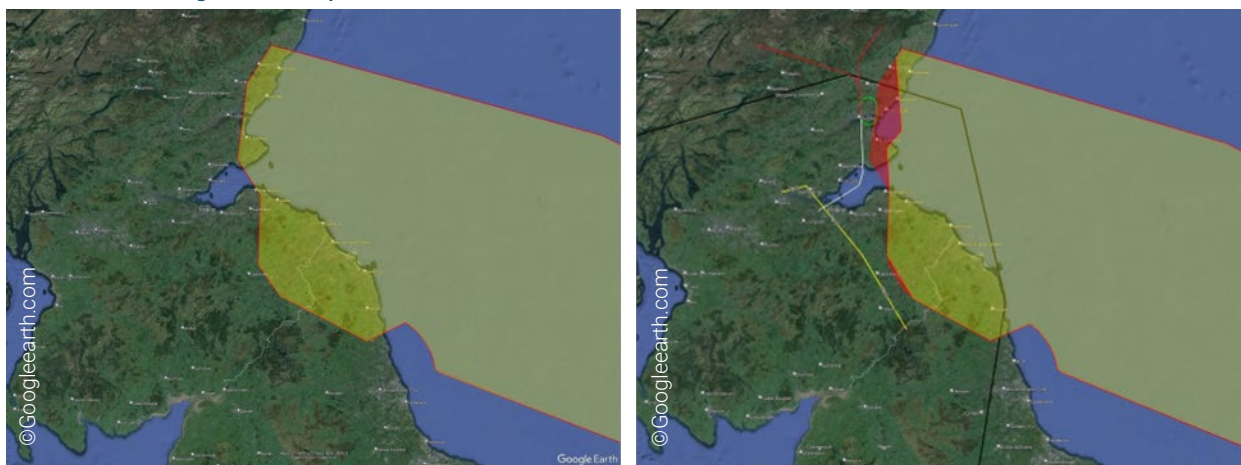
Figure 46: The extant D514 structure (in yellow, left figure (as published in the UK AIP)) and the proposed D514 structure (in yellow, right figure) the deleted portion is shown in red. ATS routes are shown in yellow, STARs in red, holds in green, transitions in white and SIDs in orange.
